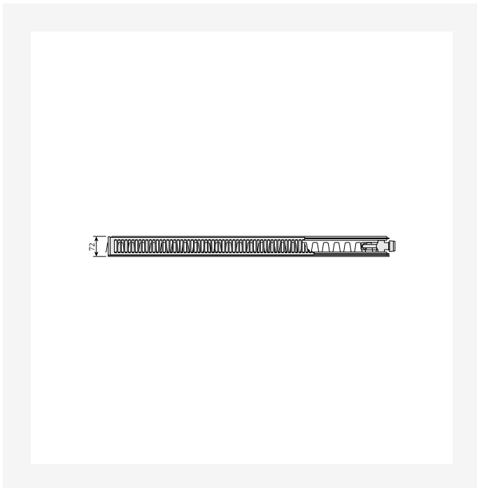
DimensionalDrawing - Plan Ventil Compact un Ramo Ventil Compact, tips 21s, pa labi, skats no augšas
