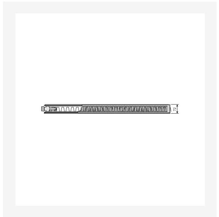
DimensionalDrawing - Plan Ventil Compact un Ramo Ventil Compact, tips 21s, pa kreisi, skats no augšas
