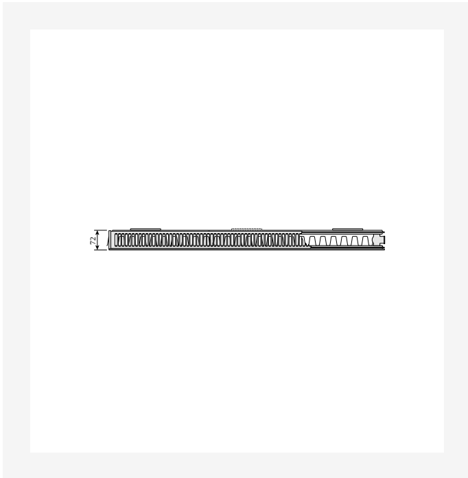
DimensionalDrawing - Plan Compact / Ramo Compact, type 21s, set oppefra
