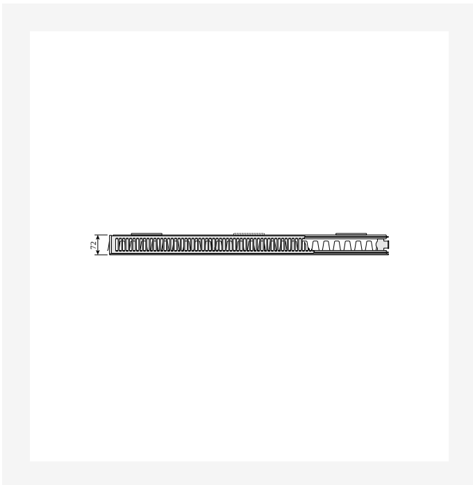
Dimensional Drawing - Plan Compact, Ramo Compact type 21s, top view
