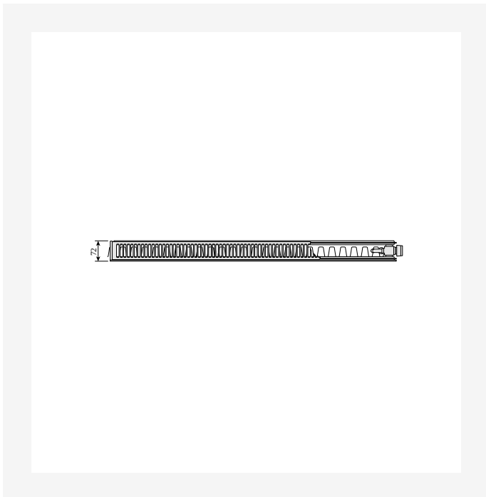
Dimensional Drawing - Thermopanel Plan and Ramo, type 21, top view
