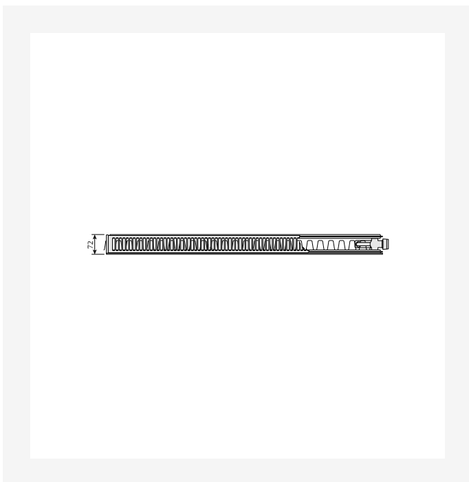
DimensionalDrawing - Plan Ventil Compact and Ramo Ventil Compact, type 21s right, top view
